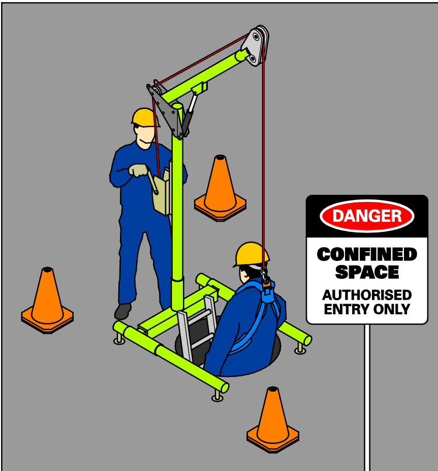
Figure 7: Standby person monitoring the confined space with rescue equipment and sign in place
