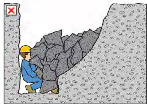
(d) Worker badly injured and probably smothered after being crushed against the opposite wall by the collapsing ground. The weight of a wedge of sand over a one metre length of trench two metres deep is about three tonnes
