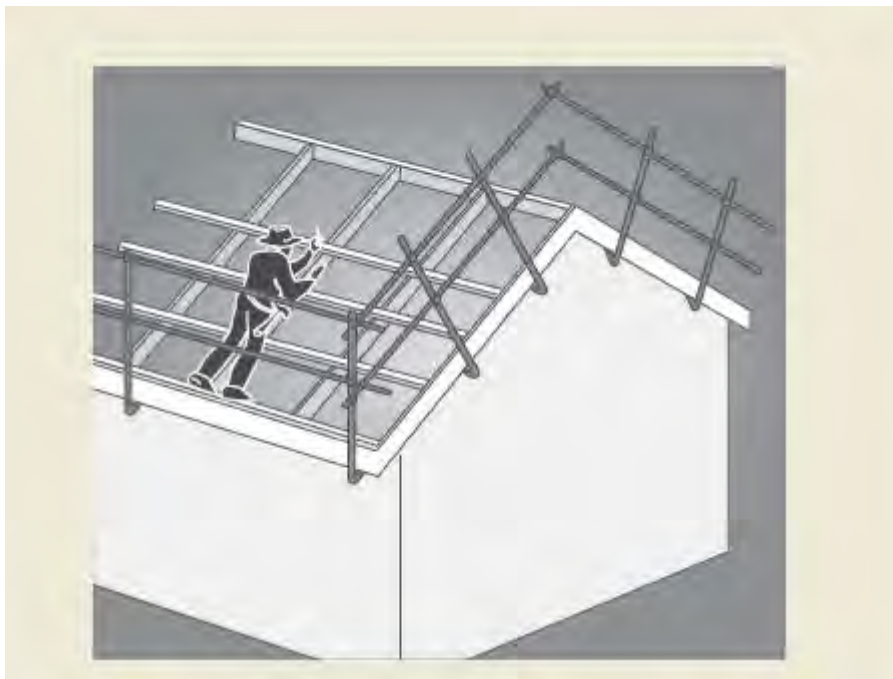
Figure 21: Fixing roof battens to trusses
