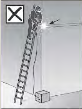
Performing hot work from a ladder
