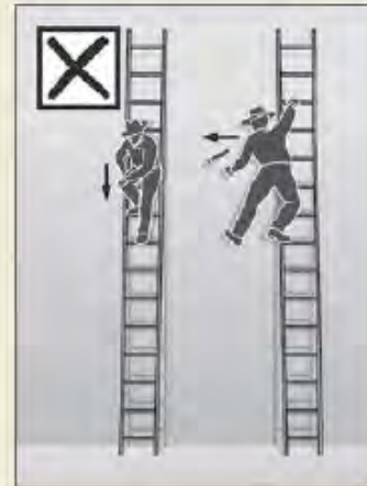
Facing away from the ladder to descend: over-reaching
