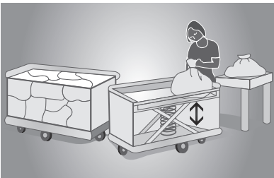
A self-adjusting base in the laundry tubs reduces the need for bending, twisting and reaching during unloading.
