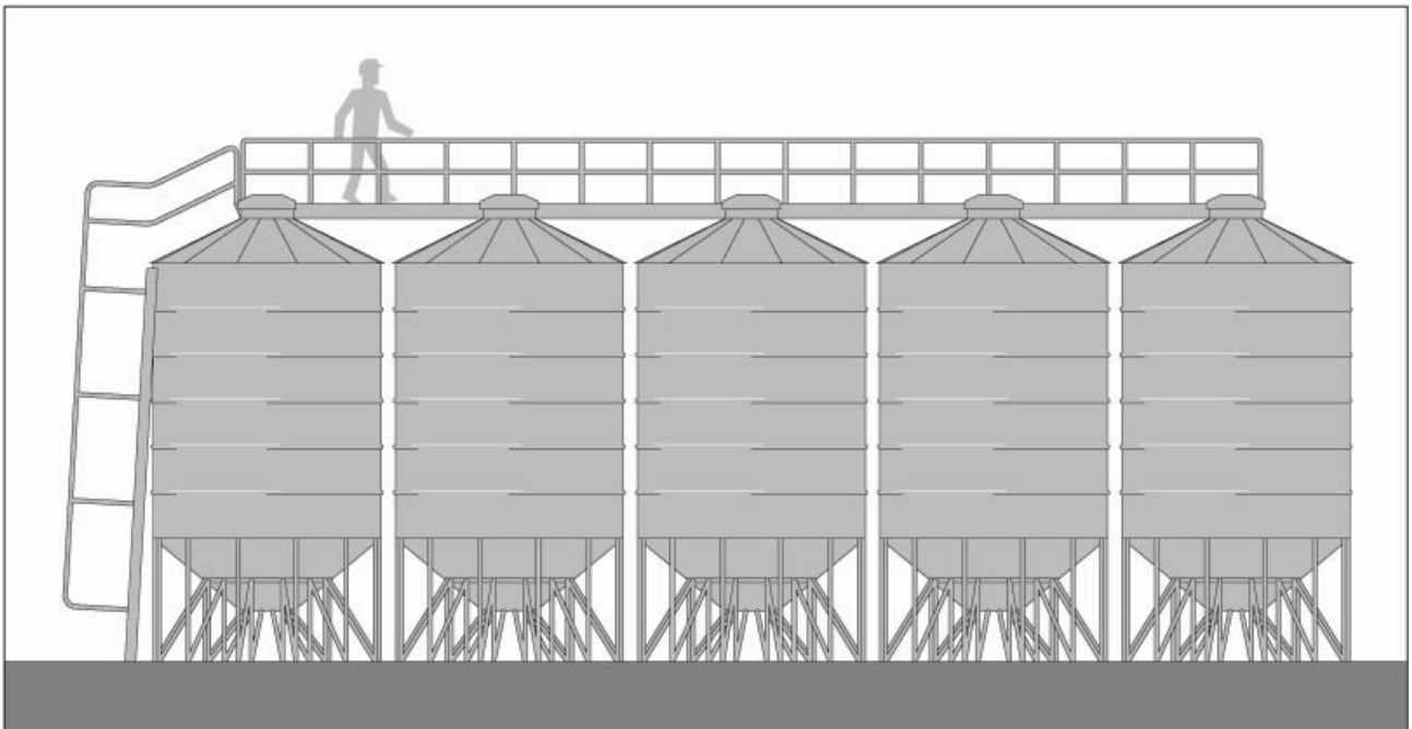
Figure 3: A platform with guard rails installed above silos
