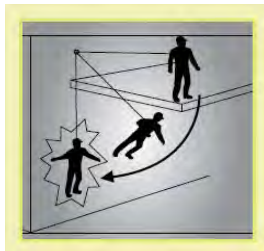
Figure 24: During 'swing back' the length of the lanyard and positioning of the anchor contact may allow the worker to hit the structure.
