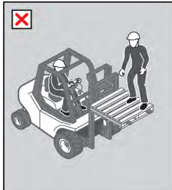
Figure 13: Using a forklift as a working platform or to gain extra height by standing on the tynes or a pallet is an unacceptable practice.
