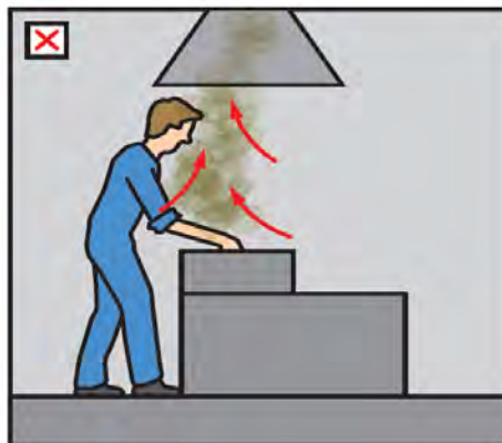
Diagram 5: Poor design carries contaminants through the breathing zone
