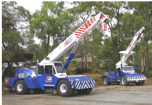
Figure 5 – Pick-and-carry mobile cranes (non-slewing hydraulic cranes)
