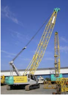
Figure 6 – Lattice boom crawler crane
