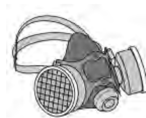
Figure 6: Half-face, particulate filter (cartridge) respirator.
