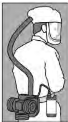
Figure 9: Full-face, powered air-purifying particulate respirator.
