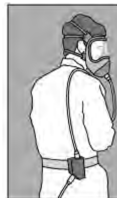
Figure 10: Full-face, positive pressure demand air-line respirator.
