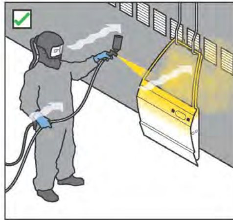
Figure 2: To avoid overspray, the article should be rotated rather than the operator spraying against the airflow.
